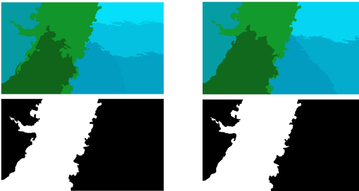
Image 7 – Resultant black and White image after applying all three techniques (SLIC, color mapping and thresholding). Number of segments is 7 for the first and 9 for the second image.
